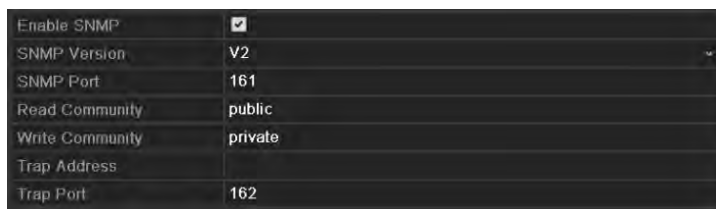
Figure 9. 16 Configure SNMP Settings
