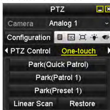
Figure 4. 11 PTZ Panel - One-touch
