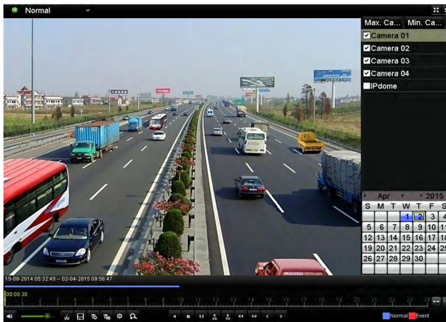
Figure 6. 9 Interface of Playback by Time
