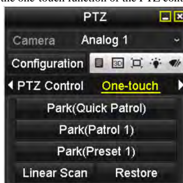
Figure 4. 12 PTZ Panel - One-touch
