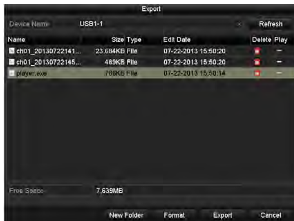
Figure 7.17 Checkup of Video Clips Export Result Using USB Flash Drive
