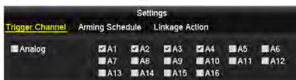
Figure 8.3 Set Trigger Camera of Motion Detection
