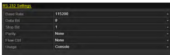
Figure 13.1 RS-232 Settings Interface
