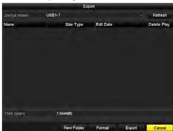
Figure 7. 15 Export Video Clips Using USB Flash Drive
