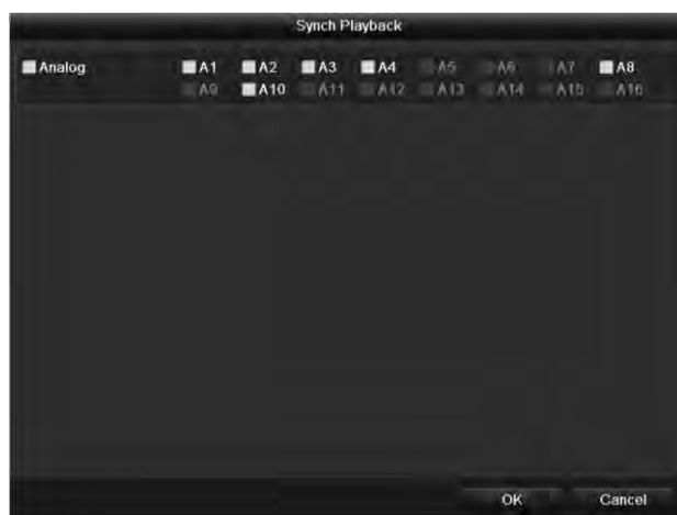
Figure 6. 7 Select Channels for Synchronous Playback
