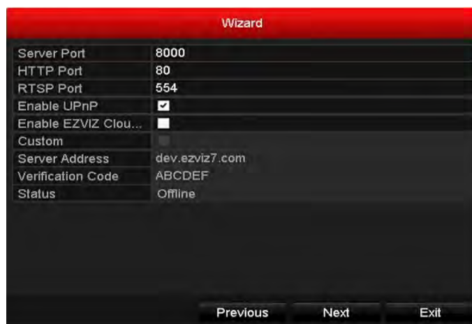
Figure 2. 8 Advanced Network Configuration
