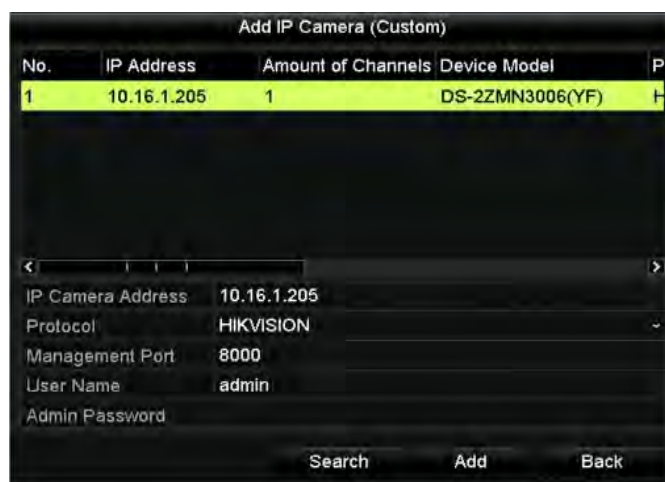
Figure 2. 20 Custom Adding IP Camera Interface
