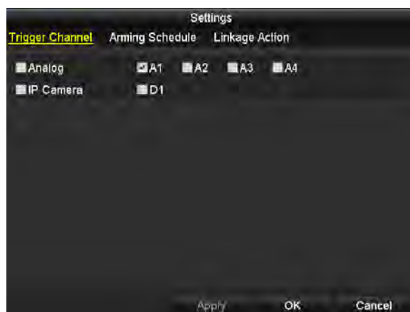
Figure 8.15 Set Triggering Channel of VCA Alarm
