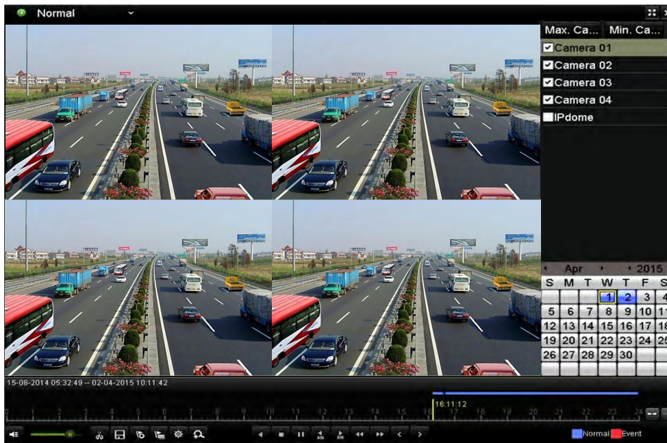
Figure 6. 19 4-ch Synchronous Playback Interface
