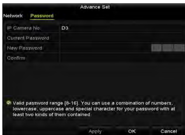
Figure 2. 24 Password Configuration of the Camera
